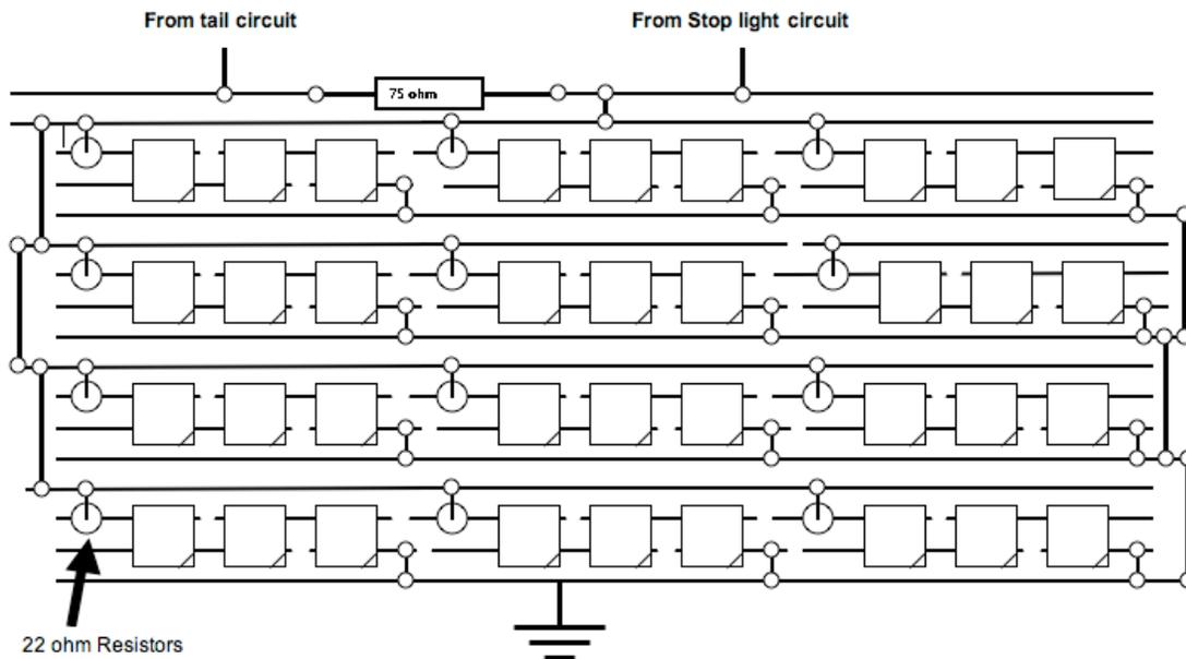
The resistors for each module are 22 ohm  $\frac{1}{8}$  watt. The tail light circuit is supplied via a 75 ohm  $\frac{1}{2}$  watt resistor, dimming the LEDs to normal brightness. The stop light by-passes this resistor illuminating the LEDs at full brightness. I have chosen to run the LEDs at 95mA for maximum brightness. This is only 5mA less than their rated maximum but since the brakes are not usually on for prolonged periods I don't expect premature failures.
