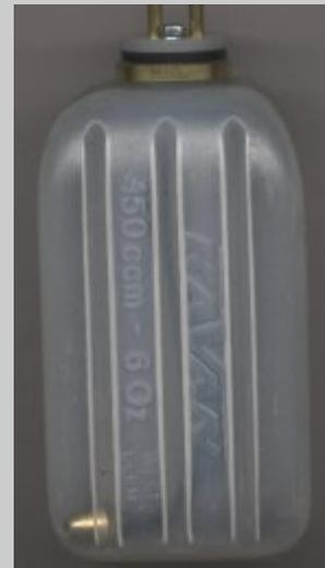
Pipes or cable straps can be led by the slots in the tank, which facilitates the safe attachment at the Mopped. Model construction catalogs offer there however still infinitely alternatives, e.g. highly polished aluminum tanks then however the factor 5-10 more expensive are.
