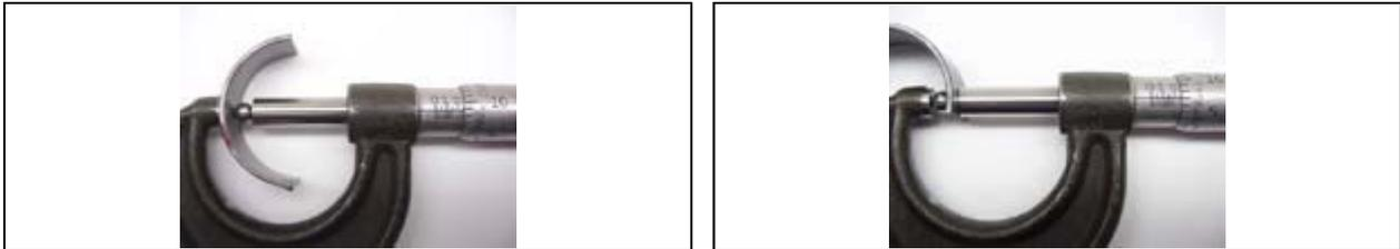
Different engines have different amounts of "bearing ovality", which is matched to the engine's RPM and the weight of its piston and rod assembly.
