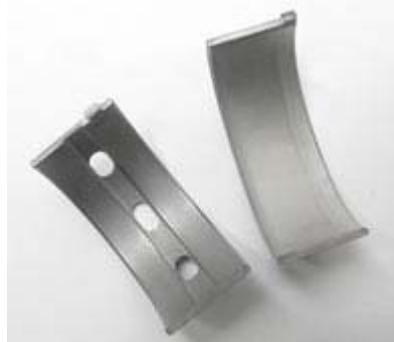
**A main bearing (left) and rod bearing (right). They just can't wait to get to work !!**
