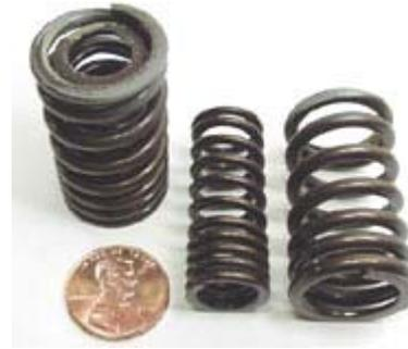
When the engine is stopped, often 1 set of valve springs are trying to push the cam forward. This force pulls up on the cam chain, which in turn pulls up on the crank.
