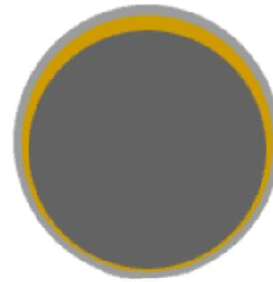
As the engine rotates, the crank journal goes "off-center" within the surrounding oil supply. Although it can move within the dimensions of the volume of oil, the crank journal surface itself never contacts the bearing.
