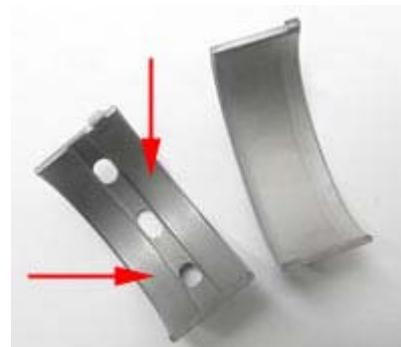
The running surface of the rod bearing is over the entire width of its surface, while the main bearing's running surface is only on the 2 outer sections indicated by the arrows.
