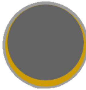
The camchain tensioned main bearing to journal relationship when the engine is turned off.
