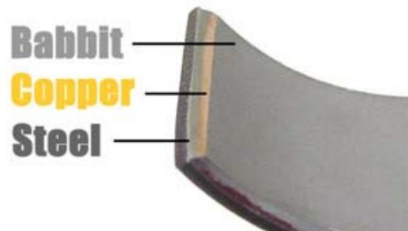
The copper layer looks thicker than it really is ... because I cut the bearing at an angle to make it easier to see the layers in the photo.
