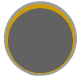
The camchain tensioned main bearing to journal relationship when the engine is running.
