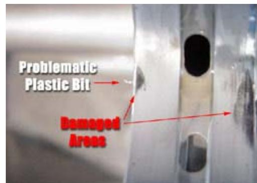
Since this bike was just removed from its crate and hadn't even been ridden yet, the damage occurred at the factory during its initial run. I first got suspicious of a problem when I smelled the faint odor of burnt oil as the crankcases were opened.
