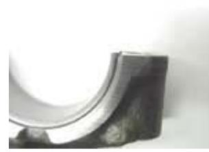
This picture of the rod's lower cap illustrates the crush concept. If you look closely, you can see that the end of the bearing insert is sticking up above the rod cap slightly.
