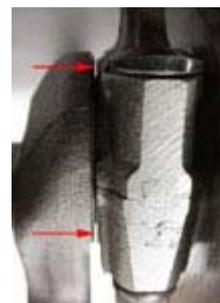
Here, I've pushed the rod to one side so it's easy to see the clearance between the rod and crank cheek.
