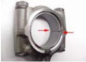
When the rod cap installed, the complete bearing is formed. In an actual engine assembly, these 2 halves are connected onto the crankshaft journal.
