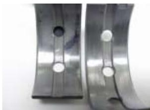
This photo shows an even better view of the cam chain tensioned main bearing's
