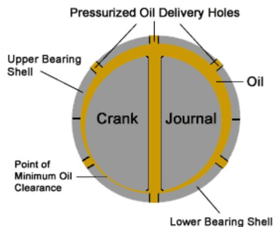
Note: As mentioned earlier, in some engines just one main bearing in the pair has oil delivery holes.
