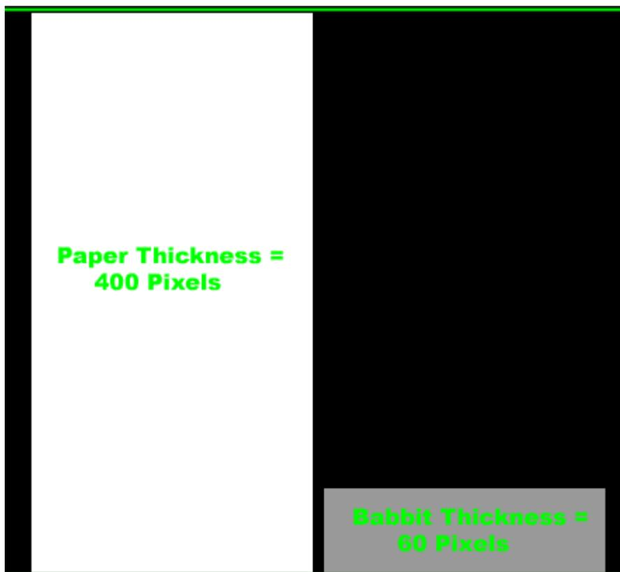
The **softest metal in an engine, the babbitt layer, is only 15% as thick as a standard sheet of paper !!**
