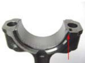
The tab on the bearing insert fits into the notch in the rod. This locates the bearing in the center of its housing.
