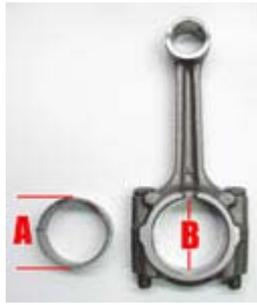
The point is that once the bearings are installed into their housing, the dimension "A" of the bearings is slightly larger than the dimension "B" of the big end of the connecting rod. (This is also true of the main bearings and the housing formed by the crankcase.)
