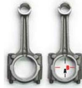
In this photo, the image of the rod on the right has been modified in Photoshop to illustrate the effect high RPM stretch has on the big end bearing's bore.
