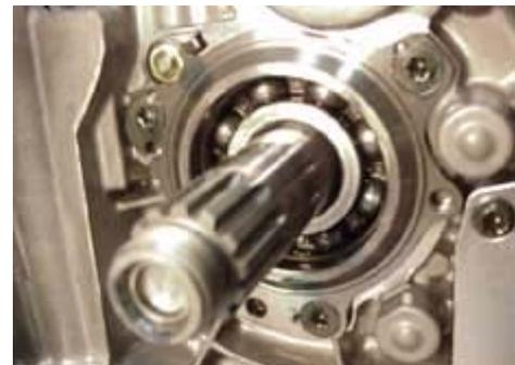
A typical ball bearing assembly used on the transmission shaft.
