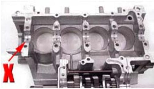
Note: this isn't a problem specific to this model, I've inspected 100's of side mounted cam chain tensioned engines from different brands and models, and this same bearing always gets worn far more than any of the others.
