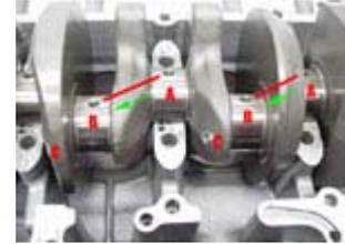
With the connecting rods removed, it's easier to see how the oil flows.
