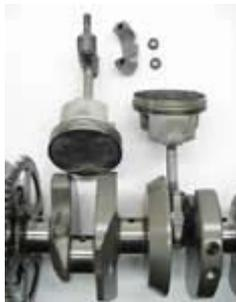
Here's how the rod connects to the crankshaft journal. The rod on the left is unassembled with the cap and nuts. The rod on the right is bolted in place.
