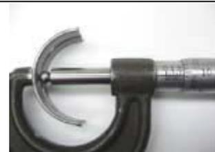
Next, measure the bearing with the babbitt layer removed ...
