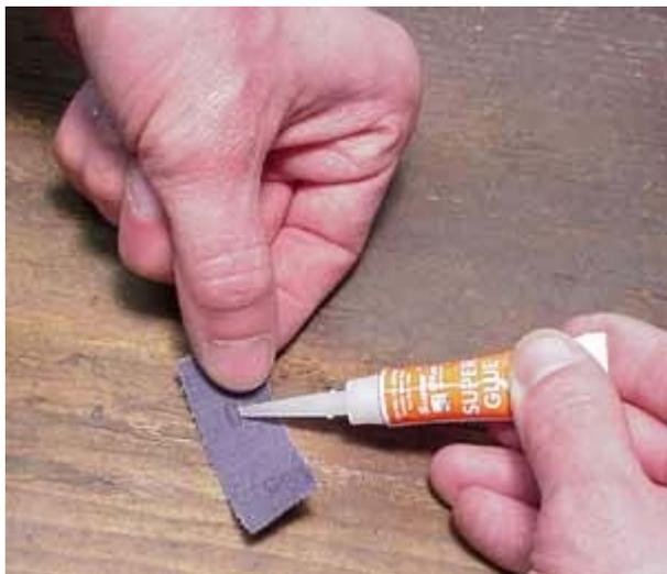
For the last step, use a drop of super glue on a piece of emery cloth...
