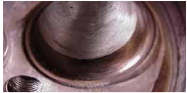
**Avoid the sealing area of the valve seat at all costs !! One nick with the porting tool will ruin the valve seal.**
