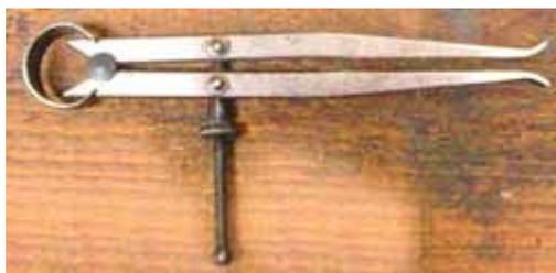
Use an inside caliper to measure the choke point...
