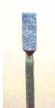
Use a thin grinding stone to get out most of the extra epoxy from around the valve seat area....
