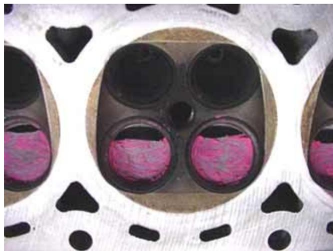
**Be SUPER careful when you're removing epoxy near the valve seat area !!**
