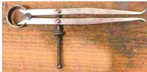
An inside caliper is used to measure the height of the tightest point in the port. This is called the choke point, and it's located between the floor downturn, and the roof of the port just before the valve guide.
