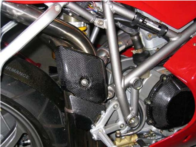
**Figure 16: Exhaust Heat Shield**
