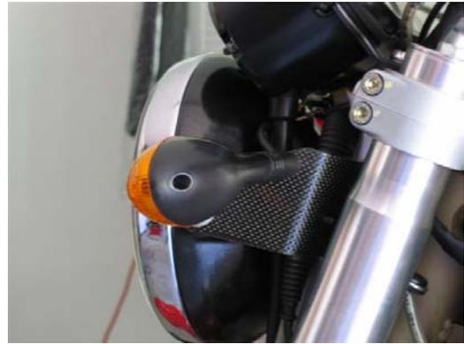
**Figure 15: Headlight Support Brackets**
