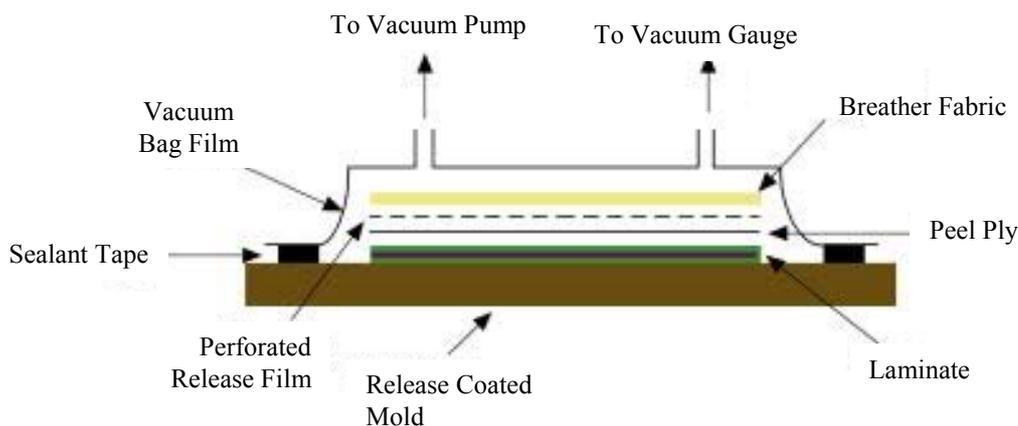
**Figure 1: Vacuum Bag Configuration**
