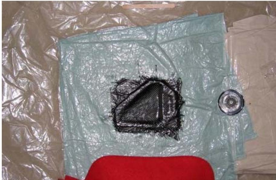
**Figure 4: Vacuum Bagged Carbon Fiber Heel Plate Layup**
