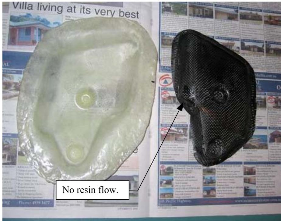
**Figure 12: Heat Shield Mold and First Attempt**
