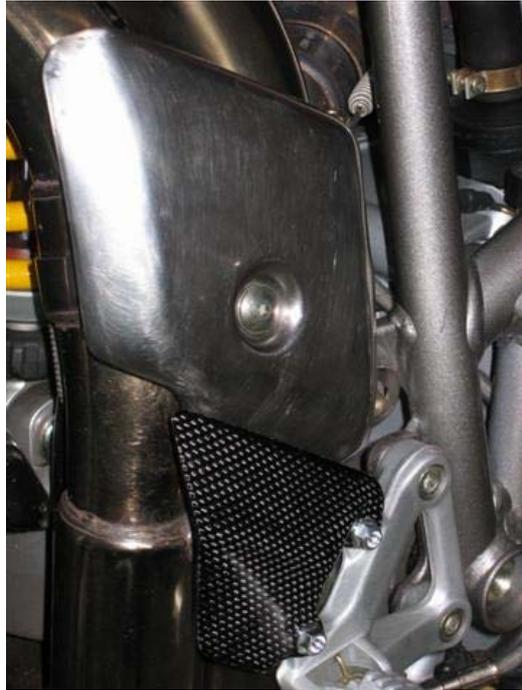
**Figure 8: 996 Rider Heel Plate - Right Hand Side**
