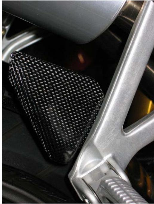
**Figure 6: 996 Passenger Heel Plate - Right Hand Side**
