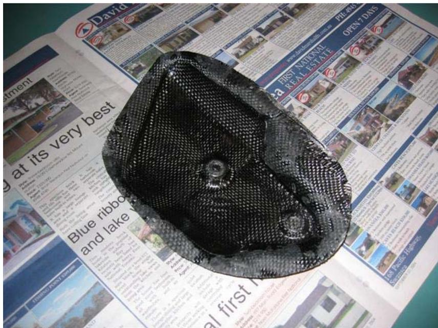
**Figure 13: Heat Shield - Second Attempt, Inside Surface**
