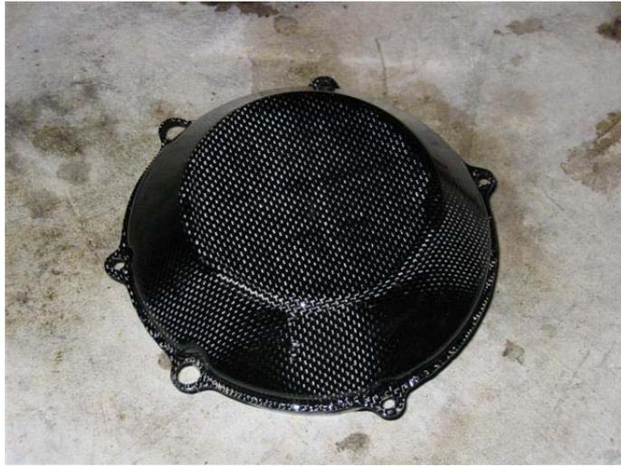
**Figure 9: Clutch Cover - Finished Part**
