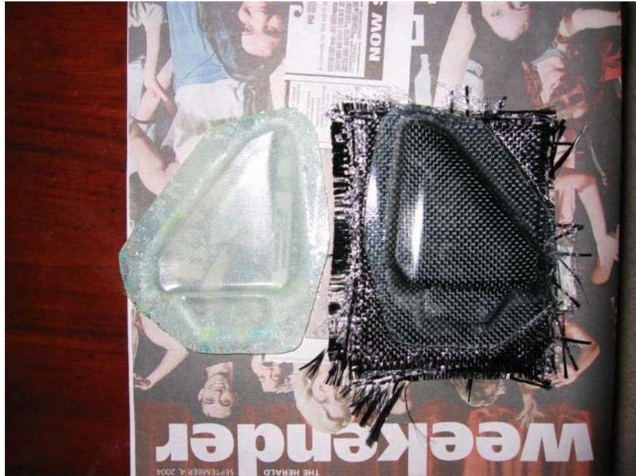
**Figure 5: Carbon Fiber Heel Plate - Prior to clean up**
