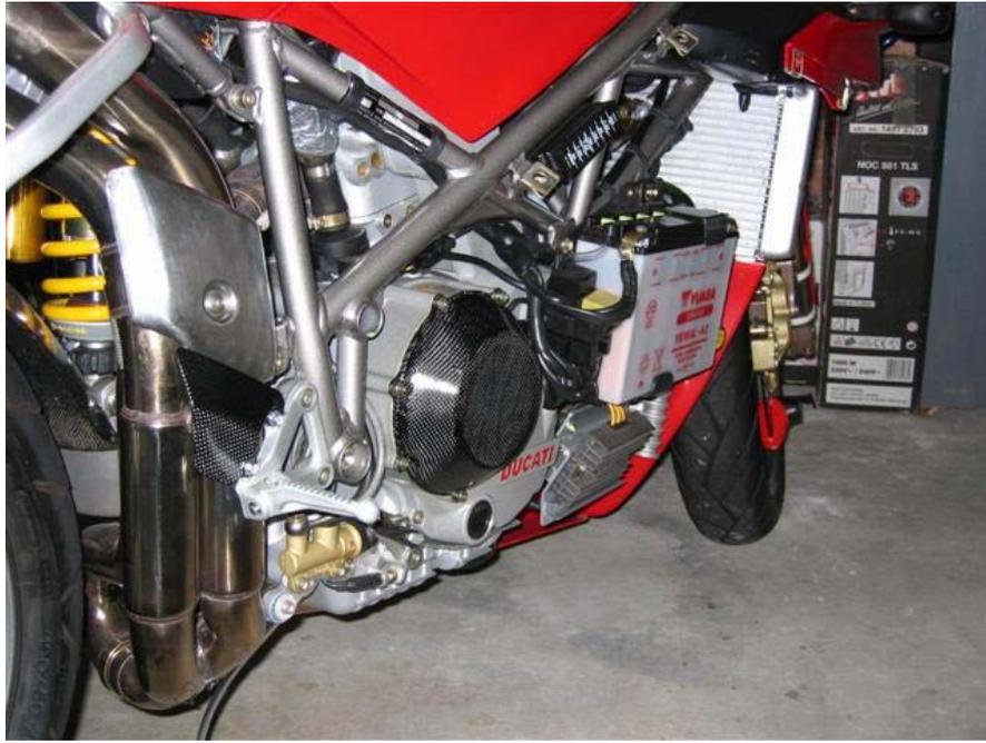
**Figure 11: Clutch Cover - Installed on Bike**
