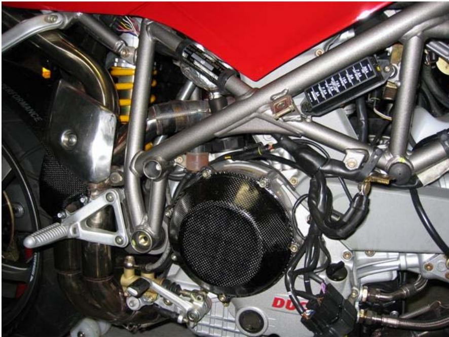
**Figure 10: Clutch Cover - Installed on Bike**
