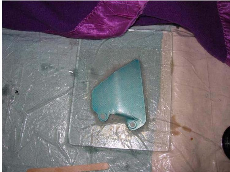
**Figure 2: Vacuum Bagged Heel Plate Molding - Rider, Right Hand Side**
